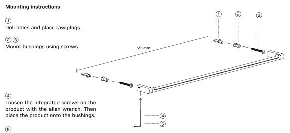
Tighten the integrated screws on the product with the allen wrench.
